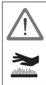
Always wear fireproof protective gloves when handling the muffler exhaust pipe extension.
